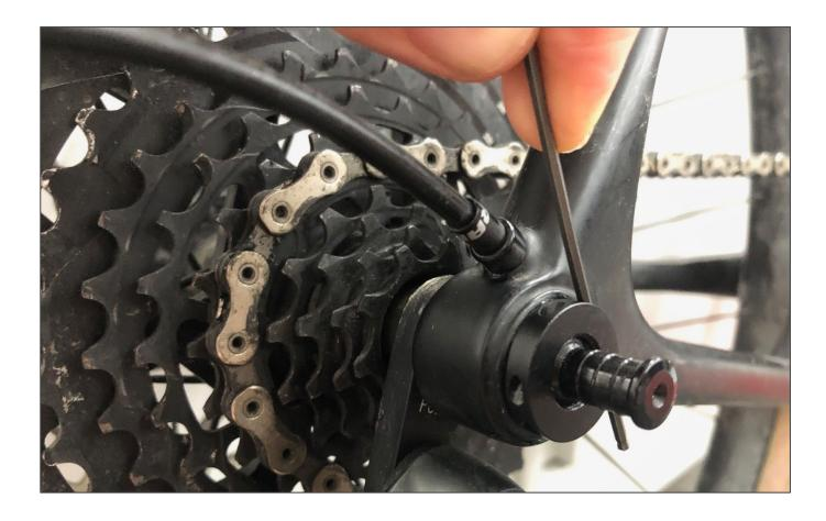
With the Axle installed attach the External locking nut and using a 2.5mm hex key (found on most multi-tools) tighten until secure.
