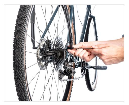
Insert correct number of spacers and screw directly to the frame
