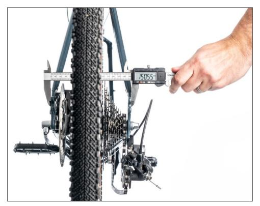
2. Depending on the width of your dropouts will determine how many spacers are required to fit the rack
