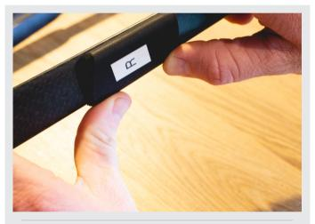
Step Five Checking the orientation of the rack, carefully select the correct left or right bumper. Now push the bumper into position, aligning with pencil mark. Ensure to limit opening the bumper as much as possible.
