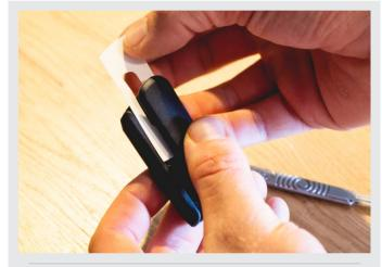
Step Three Remove the adhesive backing from the inside of the rubber bumper. Limit opening the rubber bumper. Ideally use a pin or scalpel to remove backing.
