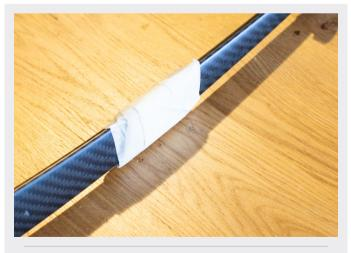
Step Six Completely wrap the bumper as **tightly as you can** using a low tac masking tape. Leave this for 48hrs to allow the adhesive to reach maximum bonding strength.
