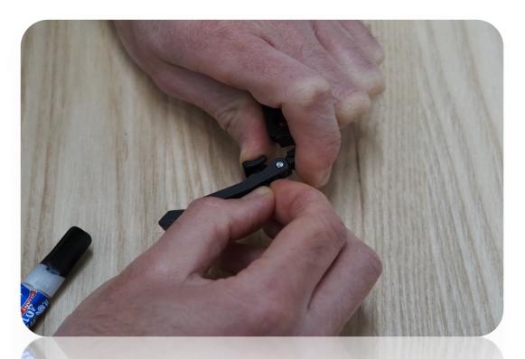
Step Four Push the bushing into the the dropout and pull on tab (Apply pressure for a few seconds for the bushing to bond)
