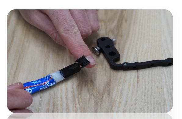
Step Two To ensure a secure fitting apply superglue to the base area of the bushing (avoid applying directly the tab)
