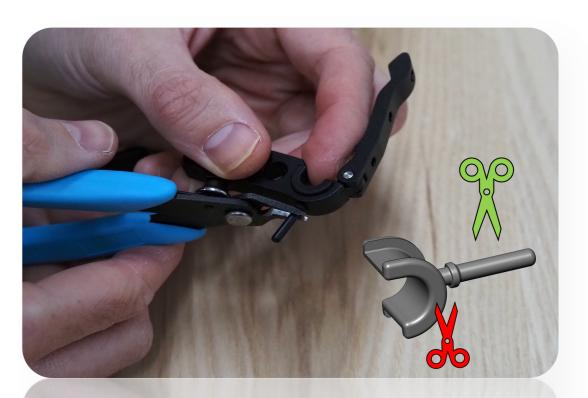
Step Five Remove the excess tab from each side of the bushing (do not cut below the tab lock)
