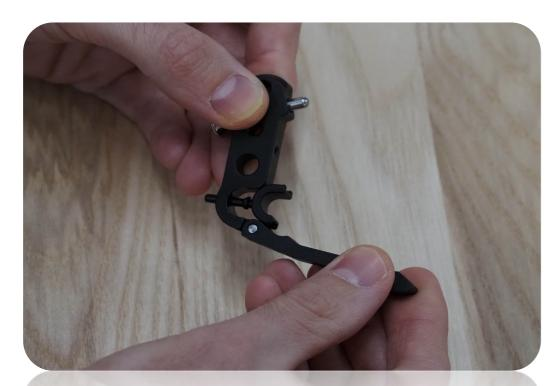
Step Three Insert bushing tab into the dropout (if having trouble pulling the tab through the dropout apply a drop of water to the tab)
